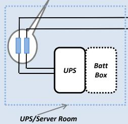
For installation and maintenance purposes, the ST4 UPS system must be installed, with at least a 1m clearence from at least three sides of the ups system
