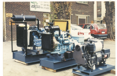
100KVA, 25KVA, 13KVA remote start/stop and AMF
